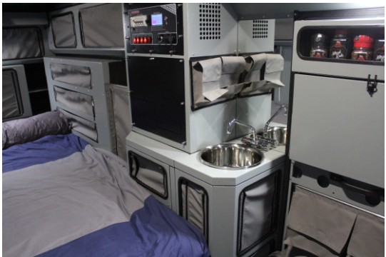
Internal stainless steel basin with instant hot water, and ample storage for toiletries.
